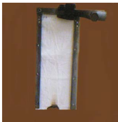
Fig. 1 Mostashari's flammability tester with a flame-retarded fabric after the end of the flammability test
